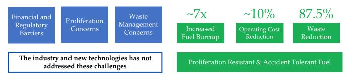
**The ANEEL Fuel Technology:** A proprietary blend of Thorium (Th) and High Assay Low Enriched Uranium (HALEU) designed for existing and new PHWR designs from Canada and India
